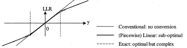
Fig. 3. LLR conversion schemes in case of considering perforation.
