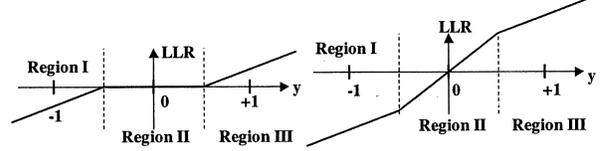
Fig. 2. Linear LLR conversion in case of considering perforation.
