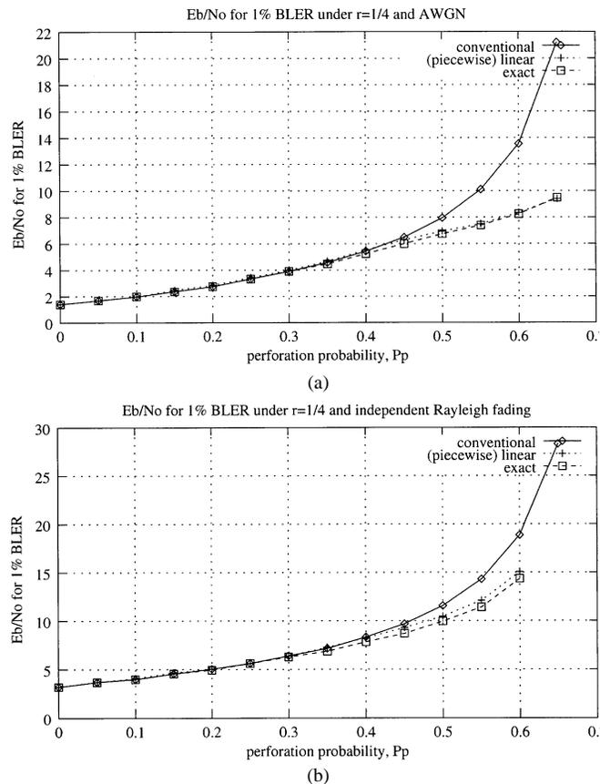
Fig. 4. Required  $E_b/N_0$  for a 1% block error rate. (a) AWGN channels. (b) Independent Rayleigh fading channels.
