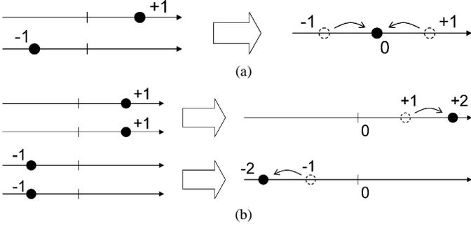
Fig. 1. Symbol mapping (BPSK). (a) Perforation. (b) Synergy with the amplitude of two symbols.
