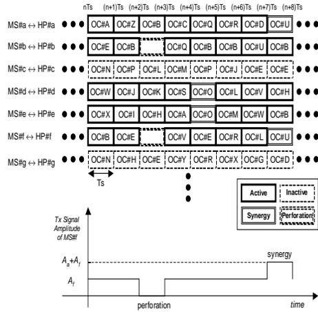
Fig. 5. Downlink Transmission Signal for MS#f
