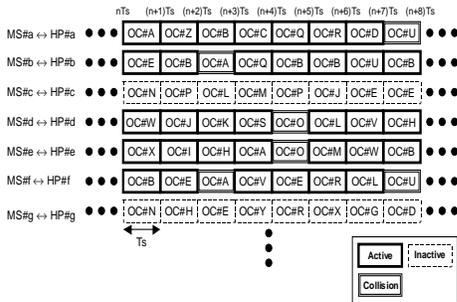
Fig. 3. Orthogonal Code Hopping Multiplexing (OCHM)
