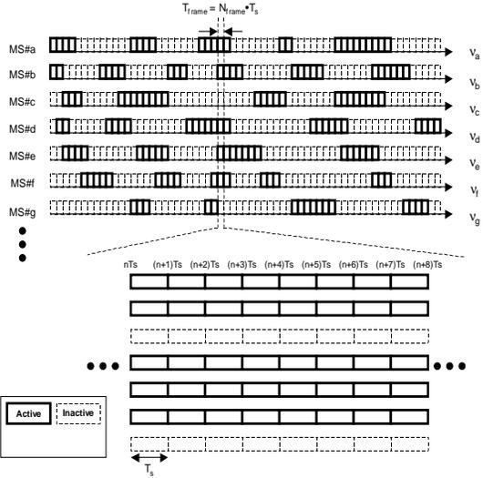
Fig. 1. Synchronous and Bursty Orthogonal Downlink Channels
