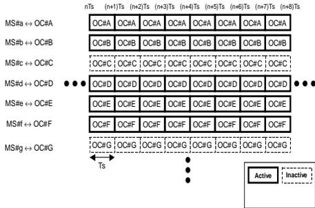
Fig. 2. Orthogonal Code Division Multiplexing (OCDM)
